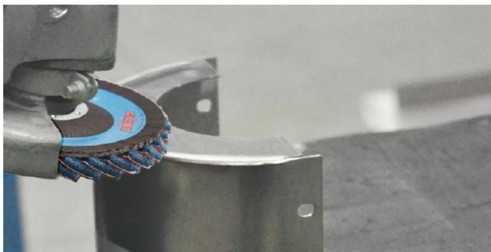
Comparisons of cleaning and polishing of weldings on stainless steel tube: before and after.
