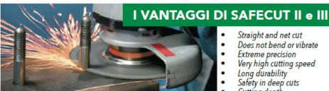
Flush cut possible thanks to the depressed center shape and the use of the "SPACER".
