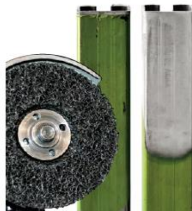
Before (SN) and after (DX) SCRUBBER pass.
